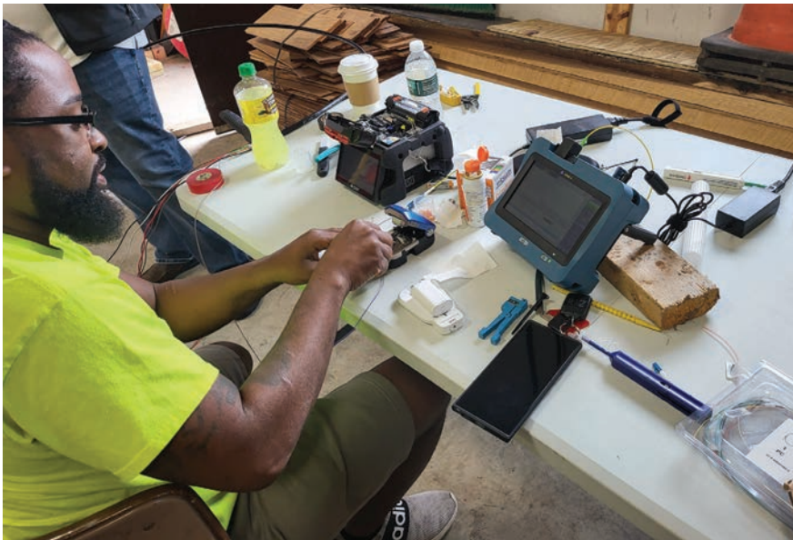
Left: Clinton trims the fiber ends prior to splicing a test end. Right: Sumitomo Fusion splicing machine.
