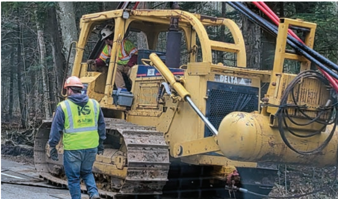
KS vibratory cable plow arriving on the Madonna (truck driver and operator's first time on a ferry), and at work below.
